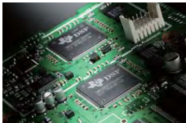
DSP unit for Transmit and Receive TMS320C6726B (Top in photo) Internal clock speed: 266MHz 32-bit floating point DSP Maximum performance =1600MFLOPS
