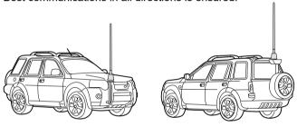
Recommended installation options on a typical pickup vehicle use a Universal Gibbet Mounting System (front) and a customer provided bracket (middle). Both methods provide effective communications in all directions.
