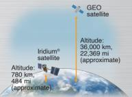
Using 66 Low Earth Orbit (LEO) Iridium<sup>®</sup> satellites, the IC-SAT100/M provides low-latency communication, and broader, more reliable network coverage, compared to Geosynchronous Equatorial Orbit (GEO) satellites.
