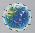
The Iridium<sup>®</sup> satellite network covers the entire globe, including both poles, and can provide global communications anywhere on the planet<sup>\*1</sup>.
