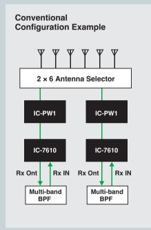
Multi-band Band-Pass Filters (BPFs) are used to prevent cross-band interference between your two radios during SO2R operation.
