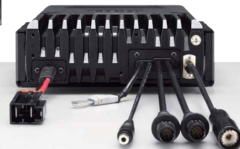
Optional CFU-F8100 fitted to the rear panel.
