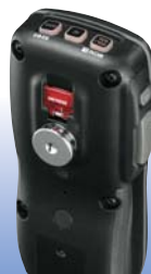
"Distress" button on the back of the unit
