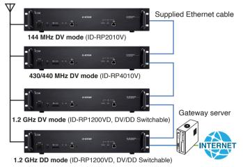
Up to 4 modules can be connected to one gateway server. The DD mode repeater must be directly connected to the gateway server.
