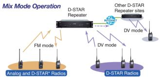
\* D-STAR radio can receive both FM and DV mode signals.
