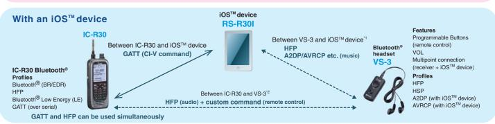
The application does not output the audio received by the receiver. The VS-3 plays either the \*1 or \*2 audio, and stands by on the other line.
