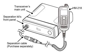
**NOTE:** Refer to the RMK-5's instruction manual for details on connecting the microphone to the separation kit.
