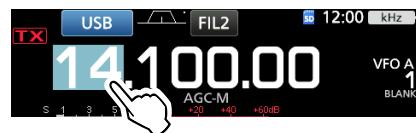
• Opens the BAND STACKING REGISTER screen.
