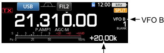
The offset between transmit and receive while holding down **XFC**.
