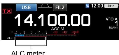
6. Adjust the MIC GAIN (p. 3-10) to where the ALC meter reads within the 30 to 50% range of the ALC zone.
