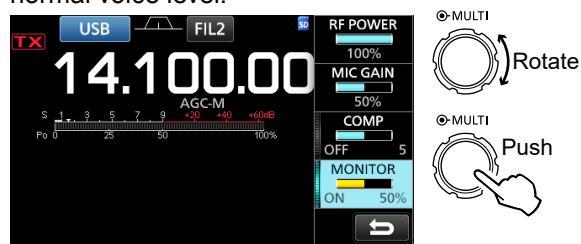
**NOTE:** When using the VOICE DELAY (p. 4-7), turn OFF the Monitor function. Otherwise the transmitted audio will echo.
