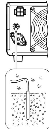
For best results, connect a heavy gauge wire or strap to a long ground rod. Make the distance between the [GND] terminal and ground as short as possible.
