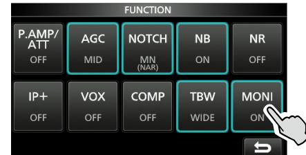
5. Adjust MONITOR to the clearest audio output between 0% and 100%, while speaking at your normal voice level.
