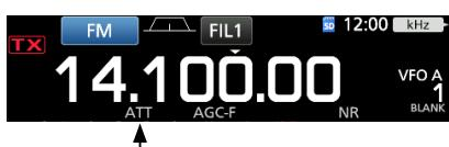
Displayed when the Attenuator is ON
