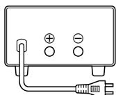
Use a power supply with 13.8 V DC output and a current capacity of at least 21 A.
