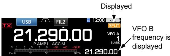
3. While holding down **XFC**, set the operating frequency offset between transmit and receive.
