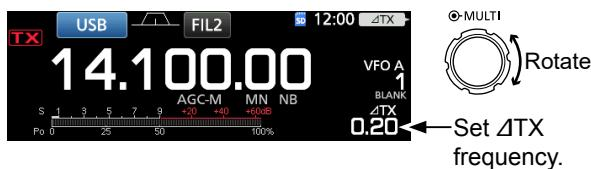
① To reset the ΔTX frequency to "0.00," hold down **CLEAR** for 1 second.
