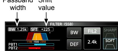
FILTER (SSB) screen (while operating Twin PBT)
