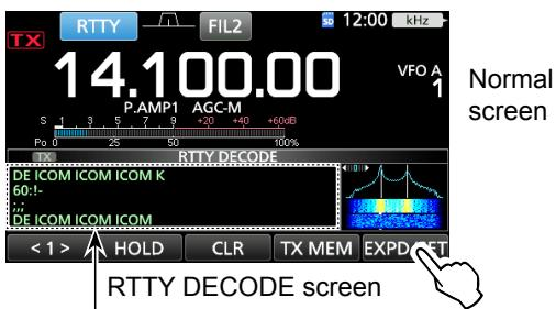
When tuned to an RTTY signal, the decoded characters are displayed.
