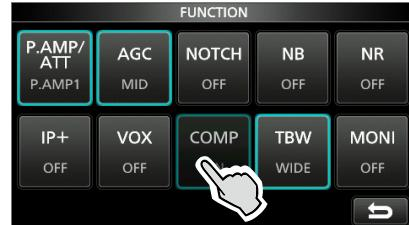
11. While speaking into the microphone at your normal voice level, adjust the Speech Compressor level to where the COMP meter reads within the COMP zone (10 to 20 dB range).
