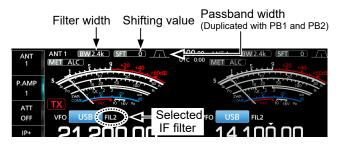
• The FILTER screen when rotating (TWIN PBT DIR)
