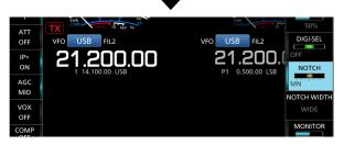
2. Rotate MULT to manually attenuate the frequency.
