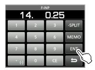
①If you touch [ENT] when the digits under 100 kHz are not entered, "0" will be automatically entered into the digits that are blank.
