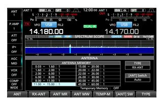
Example: Displaying the Mini scope screen while the ANTENNA screen is displayed.
