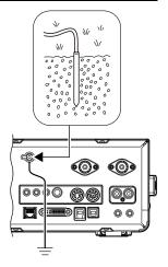
△ WARNING! NEVER connect the [GND] terminal to a gas or electric pipe, since the connection could cause an explosion or electric shock.
