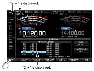
You can recall the originally saved antenna setting (Example: ANT1), touch [ANT MR].
