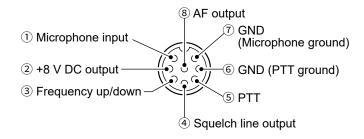
**NOTE**: Pin 1 outputs 8 V DC power for Icom microphones.
