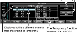
An example of antenna connector settings for each frequency band.
