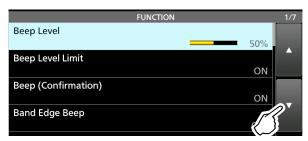
**TIP**: The Set mode is constructed in a tree structure. You may go to the next tree level, or go back a level, depending on the selected item.
