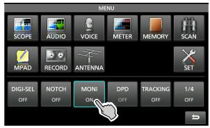
5. Rotate MULT to adjust MONITOR to the clearest audio output between 0% and 100%, while speaking at your normal voice level.
