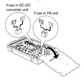
**CAUTION:** When removing a fuse, use longnose pliers to protect your fingers and the fuse holders.
