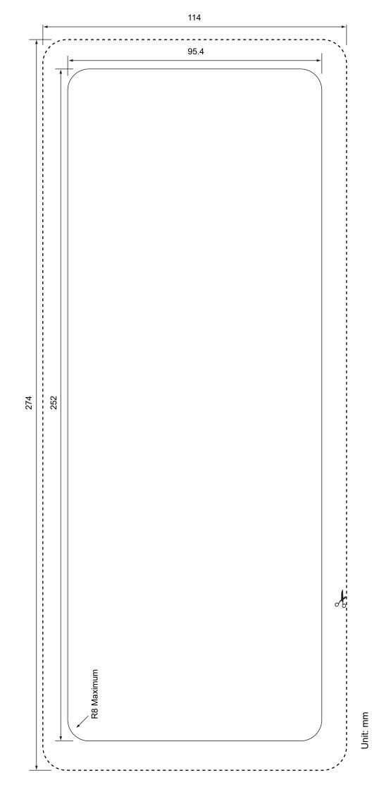
Template for flash mounting with the optional MB-75 FLUSH MOUNT KIT
