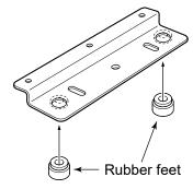
2. Attach the mounting plates to the Main unit using the 6 supplied hex head bolts (6 × 15 mm), 6 flat and spring washers, as shown below.
