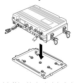
5. Lock the Main unit in place by closing the 4 latches on the mounting handles.
