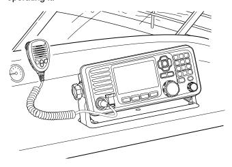
**CAUTION: KEEP** the transceiver and microphone at least 1 meter away from your vessel's magnetic navigation compass.
