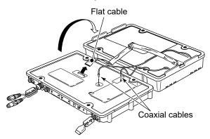
3. Unscrew the 26 screws from the shield covers, and then open the covers.
