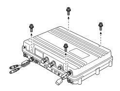
2. Open the Main unit, and then disconnect 1 flat and 2 coaxial cables, as shown below.
