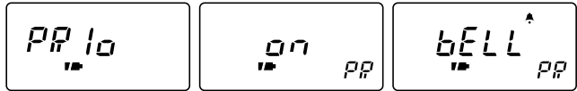
Priority watch set mode Priority watch is ON. Priority watch with alert is ON.
